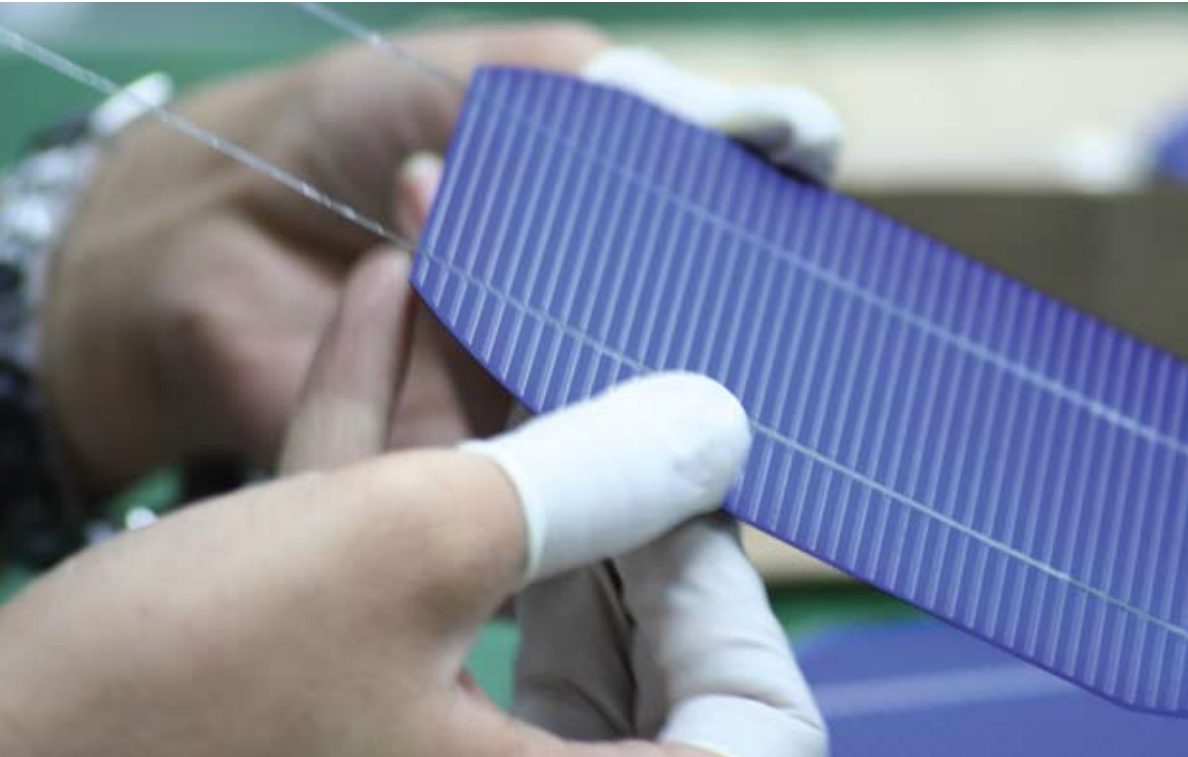
A completed solar cell, before assembly into a module (Image: Trina Solar)
